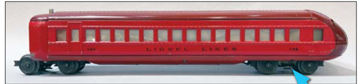
No. 794 Observation —The observation end is supported by an attached truck (blue arrow)
