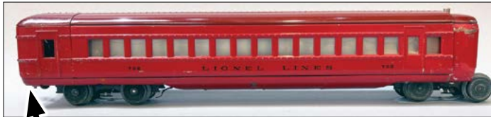
No. 792 Combine Car —Cast front (black arrow) has a scale coupler to connect to tender
